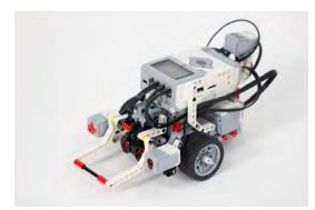
Therefore, I decided to build a "getting started" robot. It has 2 drive wheels using the large motors and a single rear wheel for support. All 4 sensors that come with the core kit are installed. This provides a platform to experiment with as I write code to activate the various sensors to direct the robot to perform various tasks. I will report on my experience next week.
